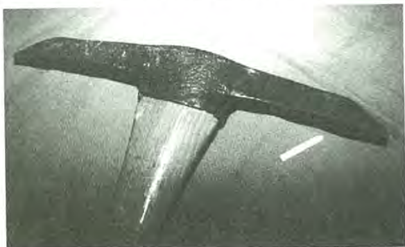
Figure 6. This drift pick was manufactured with the Bealor process. Note the ragged edge of the handle flange and crude forge-weld where its two halves were joined. The arrow points to the spot where the hardened steel tip was forge-welded onto the end of the tine. It is deformed due to blacksmith-welding and resharpening. (Author)
