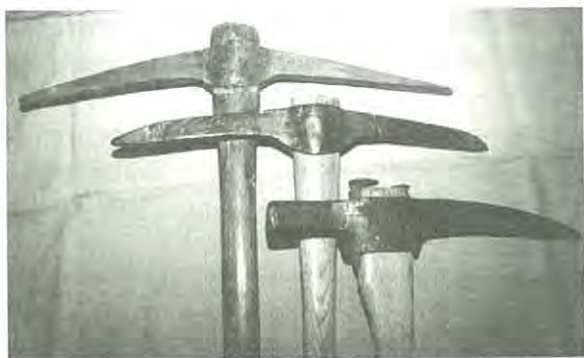
Figure 1. Top to bottom: Prospect pick, drift pick, poll pick. Two made by Collins & Co., poll pick made with Bealor process.
