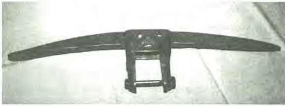
Figure 23. Note the similarity of this mechanical pick to the Eyeless model-construction is nearly identical, but it is unpatented. It probably also had interchangeable tines. The logo cast into the bracket is that of the Ames Tool Co. which operated in the early part of the 20th century. (Author)
