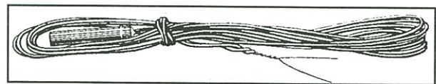
Electric cap makers usually packed their caps into boxes using the form shown in the illustration.
