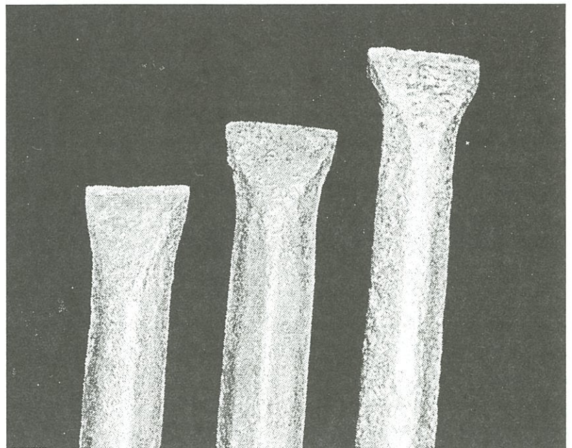
Figure 6. Set of three, 7/8 in. stock, drills found together in old workings which have straight cutting edges and no upsetting before forging. (cir. late 1890's)
