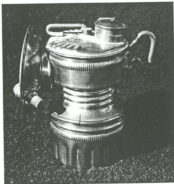
A split flange is a common problem for Droppers.
