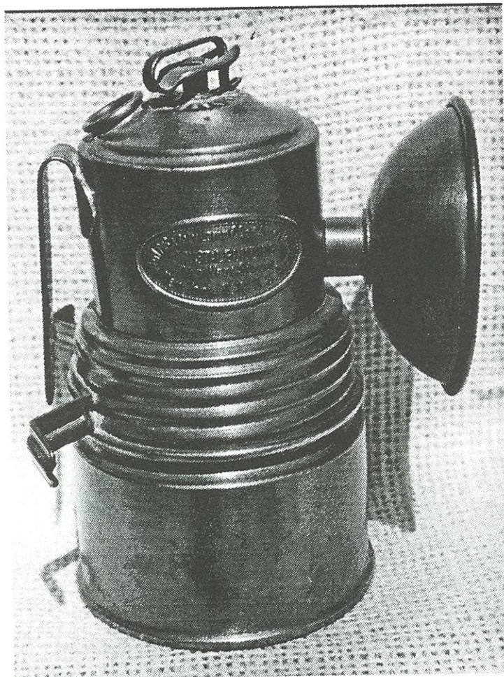
Wolf's first American made carbide cap lamp.
