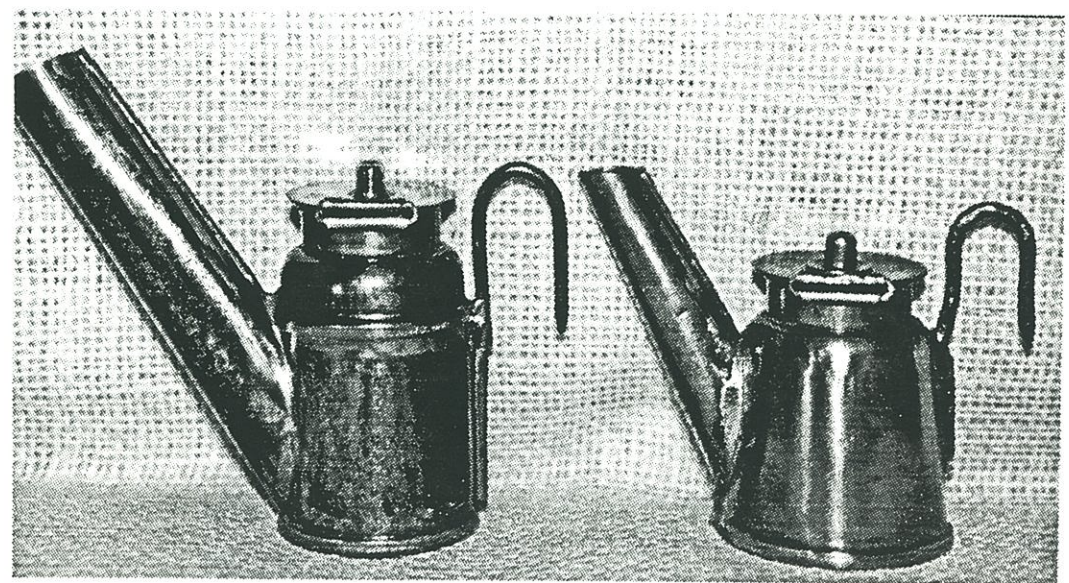
Left: tin face lamp with brass collar and cap and stamping B, G, and I.
