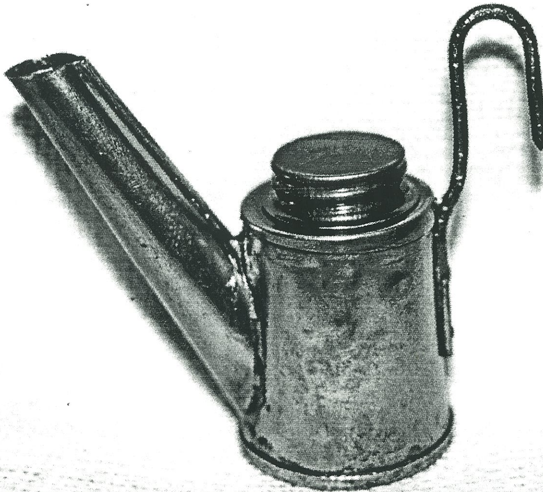
Copper Logan-Gregg with tin threaded cap.
