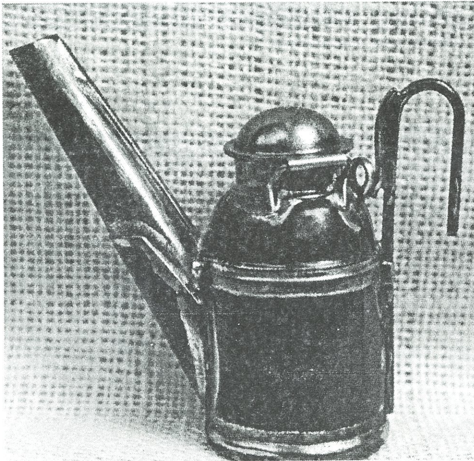
Trethaway Bros. oil wick lamp with the T.A. Black vent tube.
