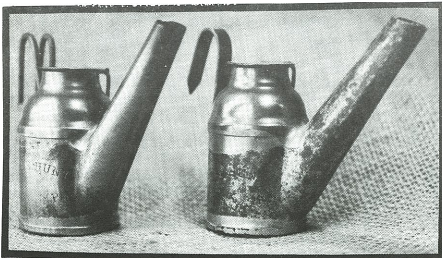
Figure 4. Oil Wick Lamps made by Alex E. Hunt of Scranton. Note the unusual double and flat hooks.
