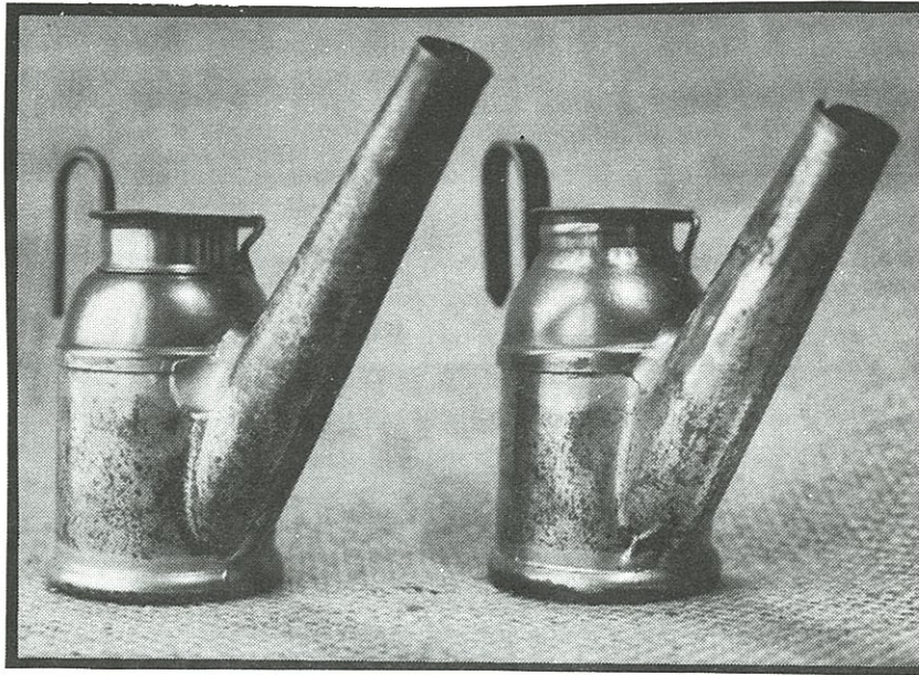
Figure 5. Oil wick lamps made by Trethaway Brothers of Parsons, Pennsylvania. The lamp on the left is marked Alex E. Hunt, while the lamp on the right with the unusual flat hook is marked Trethaway Bros.
