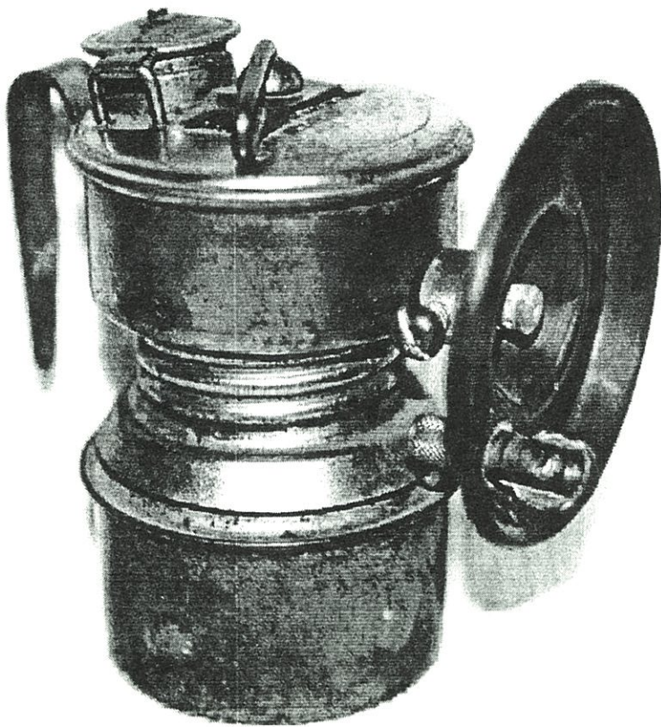
Early "One-Date" Guy's Dropper with 5-bump base and narrow spade mount (Dave Johnson collection.)
