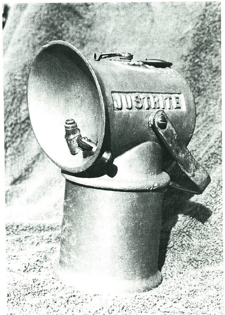
Fig. 3 Jumbo hand lamp. This variety has the low mounted burner, a conventional bail & hook, patent stamping on the opposite side, and a round spring loaded water door.
