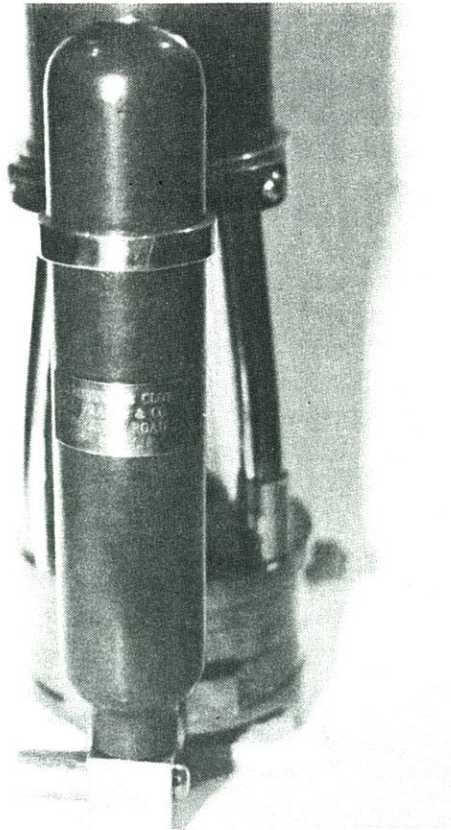
Clowes hydrogen cylinder, bearing a brass tag marked: Redwood & Clowes Patent W. J. Frasher & Co. Commercial Road East London
