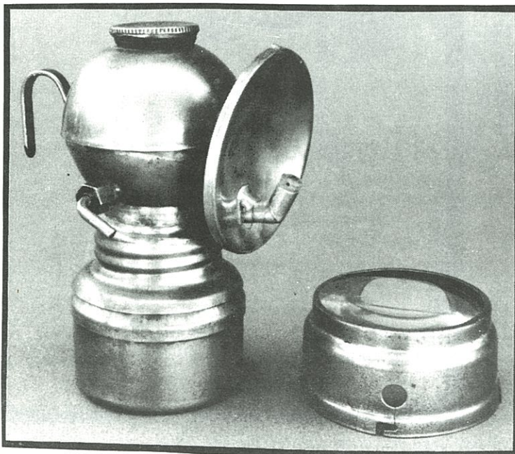
Figure 7. A photograph of the only known example of an Ever-Ready lamp with the attachable lens. (Bill Spence photo)
