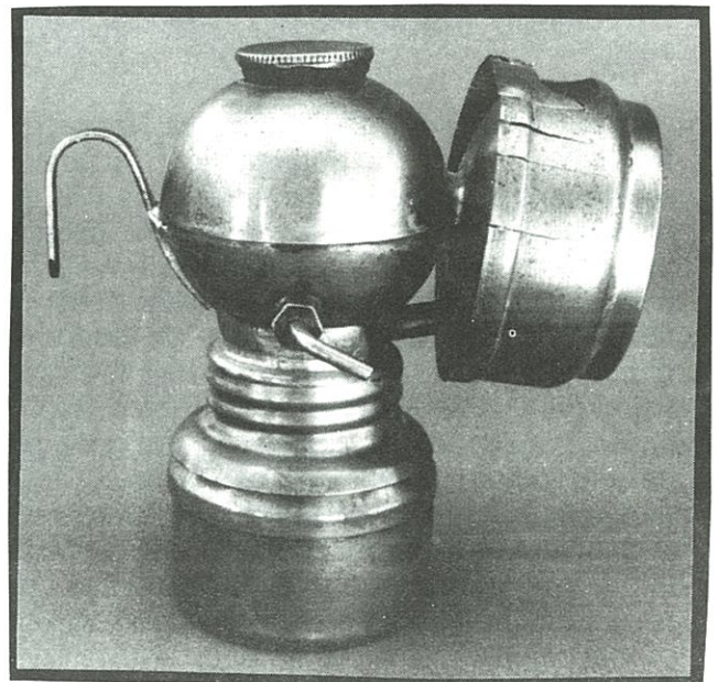
Figure 7. A photograph of the only known example of an Ever-Ready lamp with the attachable lens. (Bill Spence photo)
