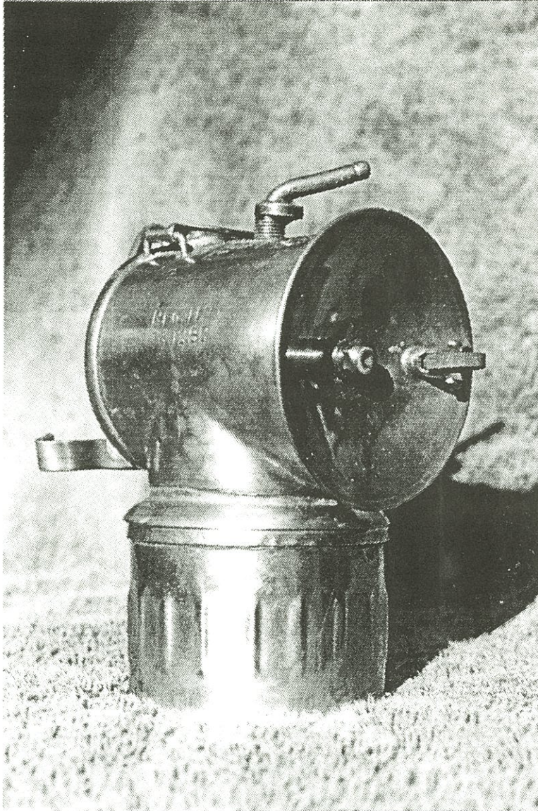
The Rex Lamp: An English copy of the horizontal Justrite. Stamping on the left side is shown below.
