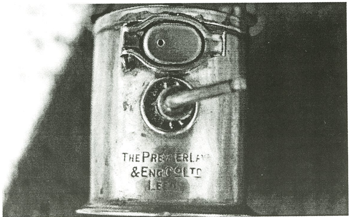
Top view shows the company stamp, oval water door, and water lever notches.
