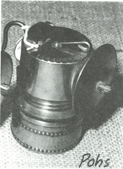
Figure 3. All brass Harker Brothers Brite-Lite with oval water door, knurled base and top mounted lever-feed. (ex Henry Pohs collection)
