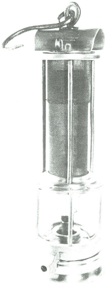
T.B. Bickerton Clanny lamp is 10 inches high, and stamped on the top. From the J. Roger Mitchell collection, photo by R. Pearl.
