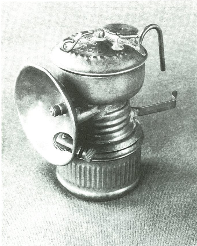
Perhaps the earliest GEE BEE cap lamp, brass, with 2 1/4" reflector. Note soldered on reflector and flat strip braces as on early Grier Bros. lamps.
