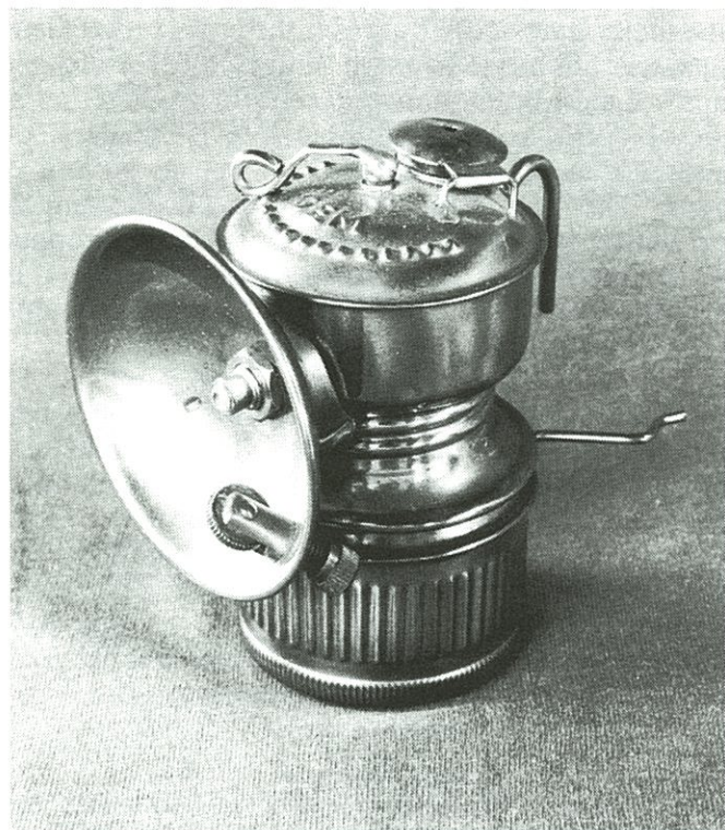
GEM cap lamp, brass, 2 1/2" reflector.
