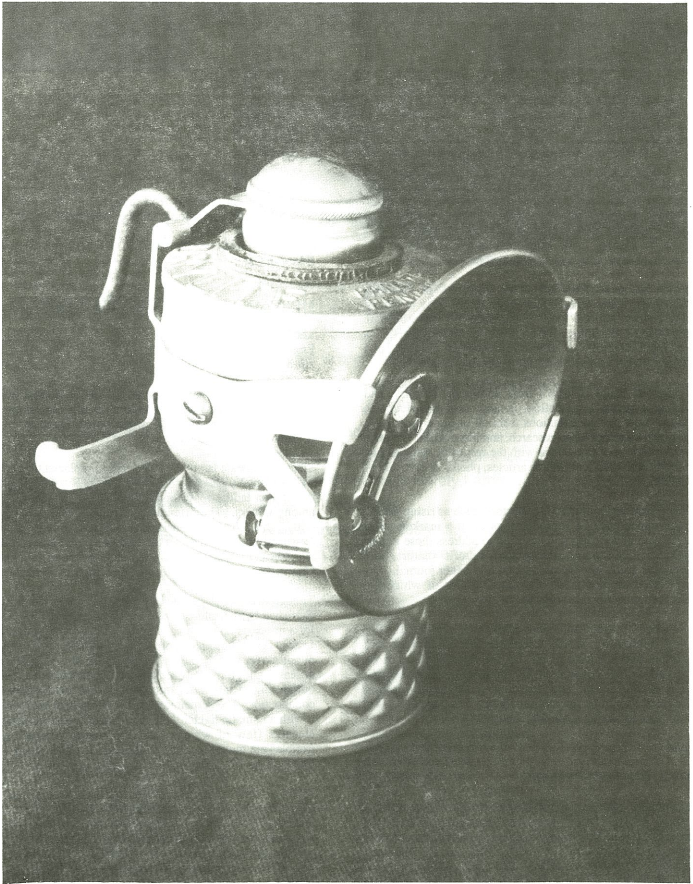
Hansen's first cap lamp: The Drylite
