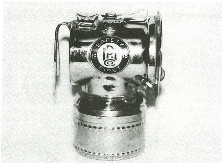
Nickel-plated Justrite cap lamp with enamel plaque, a presentation piece for safety. The lamp is equipped with the typical Michigan narrow flat hook.
