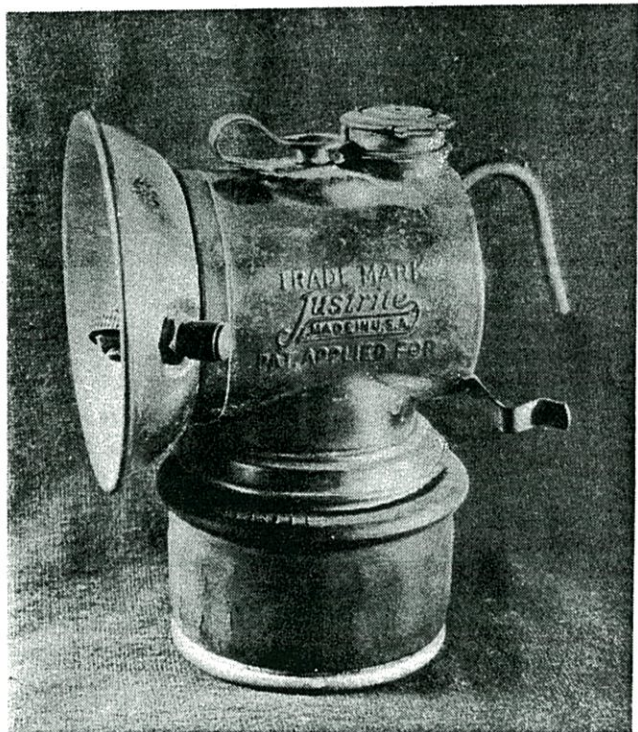
Early 1930's vintage lamp showing change to complete absence of patent dates, removable reflector, and the "Protecto-grip" base.
