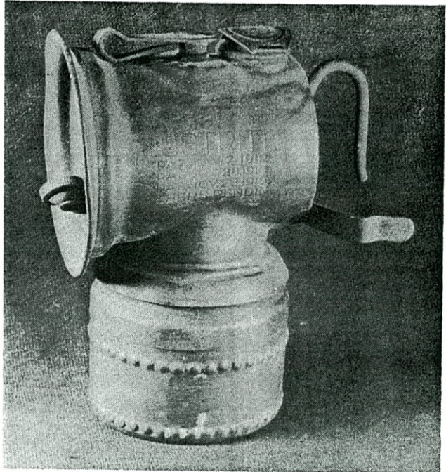
Ca. 1917 "Lever Feed" cap lamp, showing the larger lever and a revised trio of dates. (D. Thorpe collection)
