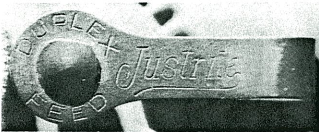
Close-up of Duplex Feed water lever (ca. 1922).
