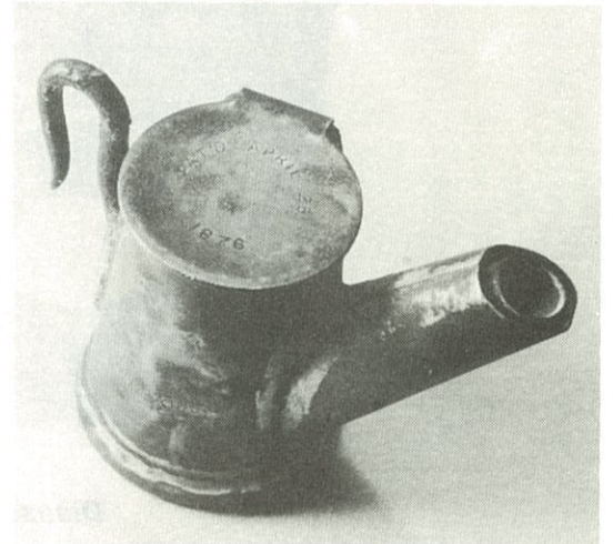
A third, and completely different Miner's Supply Co. Oil wick lamp (tin) with accompanying side stamp. Note patent date (April 25, 1876) stamped on top of door. (Bob Schroth collection)
