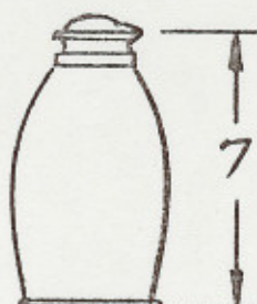
UNMARKED 1 lb Carbide Flask T. F. Leonard type Hinge from oil wick cap Lamp OVAL - STEEL
