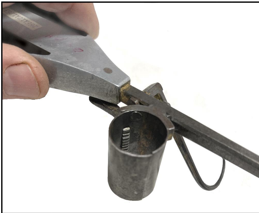
Note the grab ridges inside the thimble
