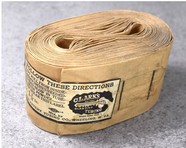
Roll of Clark Blasting Tubing. Note the printed marks to the right of the label for measuring lengths of tubing.
