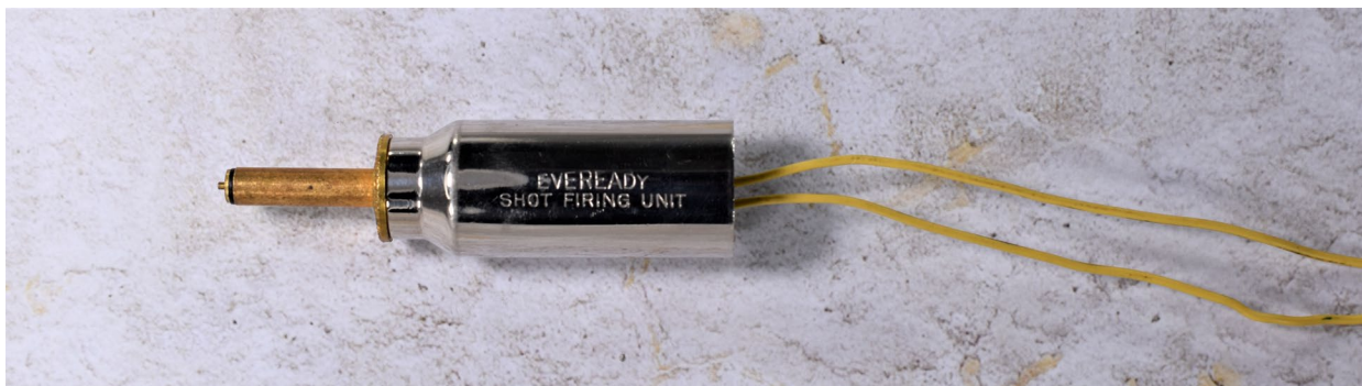
Wires were threaded through housing of the firing plug and attached to the firing pin with screws.
