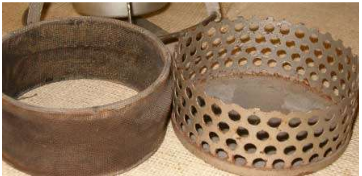
Bottom gauze removed from base.
