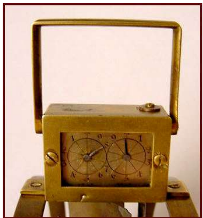
Davis Biram anemometer and closeup of dials, ca. 1845.
