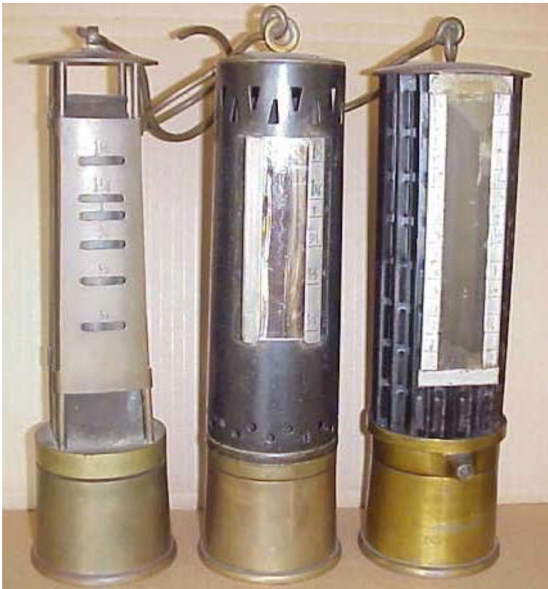
Figure 14: Friemann & Wolf No. 700, 701, &702. These are the three “classic” and most advanced models from F&W. All have igniters and flame “snuffers.”
