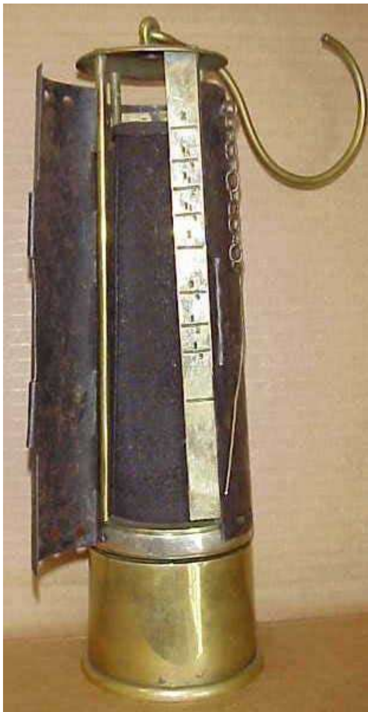
Figure 5: Friemann & Wolf Pieler. Serial No. 80643; circa 1890. This lamp shows how F&W customized lamps for particular needs. This lamp has a removable bonnet, two (2) types of observation scales, a flame snuffer and magnetic lock. From the 1880's to 1900, F&W produced Pieler lamps with many variations. After 1900, the basic F&W models were the No. 700, No. 701, and No. 702.
