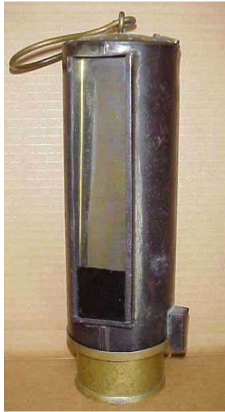
Figure 7: J. Mills & Sons Newcastle bonneted and unbonneted Pieler lamps. Pieler lamps were not popular in England as Ashworths and Clowes Hydrogen lamps were preferred. Notice the bonneted lamp has no scale, and has a painted black standard on the viewing glass. The author doubts if another English make exists.
