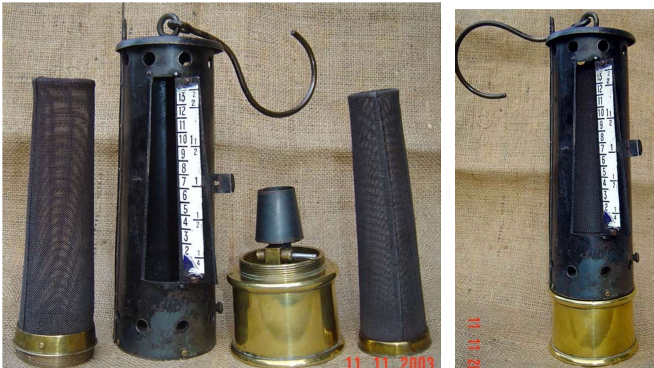
Figure 10: Belgain Mulkey Pieler. Invented in Lens, France, this particular lamp has the most sophisticated safety features of any Pieler lamp the author has seen. These features include a locking mechanism for the bonnet, double gauze arrangement, and a device to insure the gauzes have been inserted when assembling the lamp. It also has air regulators on the top and bottom of the bonnet. The scale is made of enamel.
