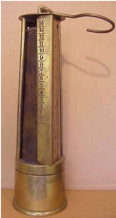
Figure 8: French Cosset-Dubrelle Pieler. Notice scale measures length in centimeters, with no % methane indication.
