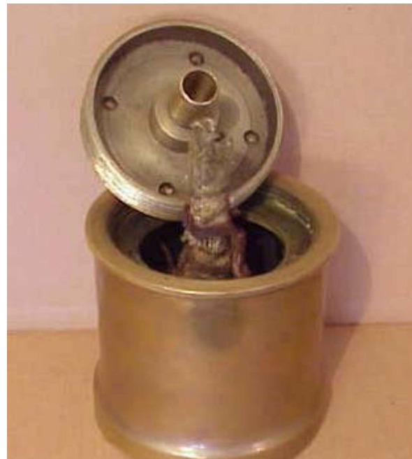
Figure 2: (above and right): This is Pieler's original design, but with scales added. The gauze is steel with a copper cap similar to a Saarbrücken lamp. The font is complex because of having to facilitate the hallow tube that runs from the bottom of the lamp through the center of the burner. Circa 1887.
