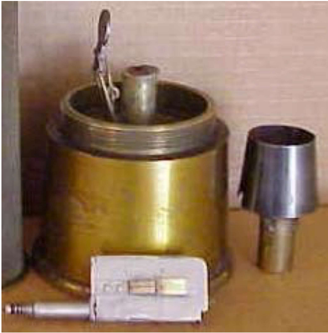
Figure 15: Friemann & Wolf. Detail of flame “snuffer” and igniter.
