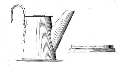
In the Fleming patent, a heavy cast disc is used for the base. This functioned like a "boot-kick." Its stiffness prevented denting of the lamps edge.
