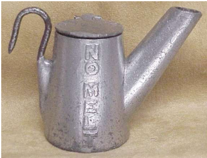
Above: The NO MELT lamp follows the 1909 Hammond Patent shown next page
