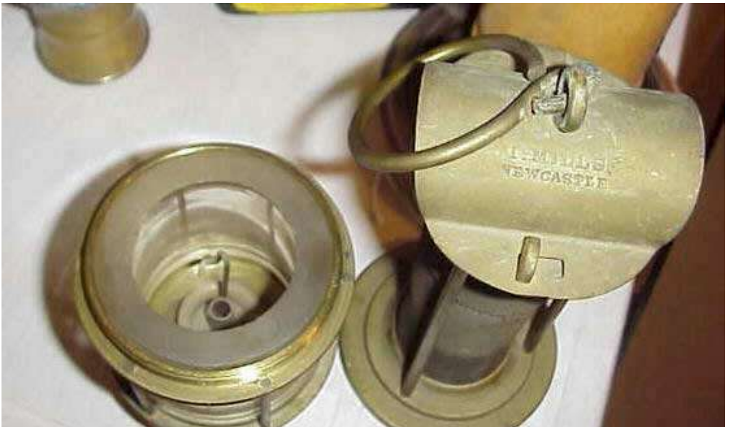
Below: the disassembled lamp reveals a very thick sight glass.
