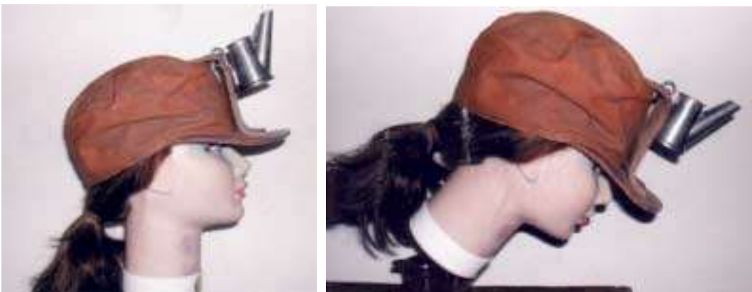
Figure 1: Standard oil wick face lamp. Note the angle of the spout in the upright and then the flexed figure. It would not take much more of a bend to allow the oil to pour from the spout.
