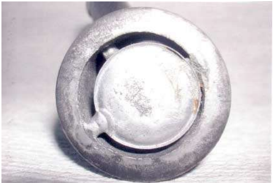
Figure 14: H. J. Richards lamp. Note the fuel chamber surrounds the wick chamber and the fuel flows through small connecting channels.
