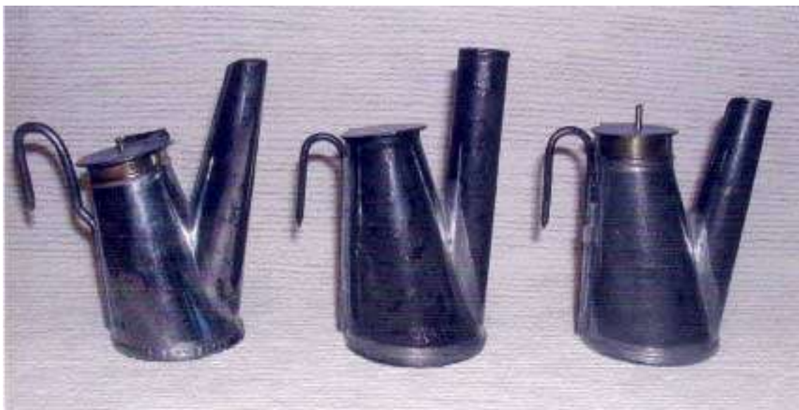
Figure 6: Three models of leanback lamps. The Felix, the P & A Good, and the Trethaway. Note the almost vertical angle of the spout of the Good lamp. Also note the bottoms of these lamps are oval, not round.
