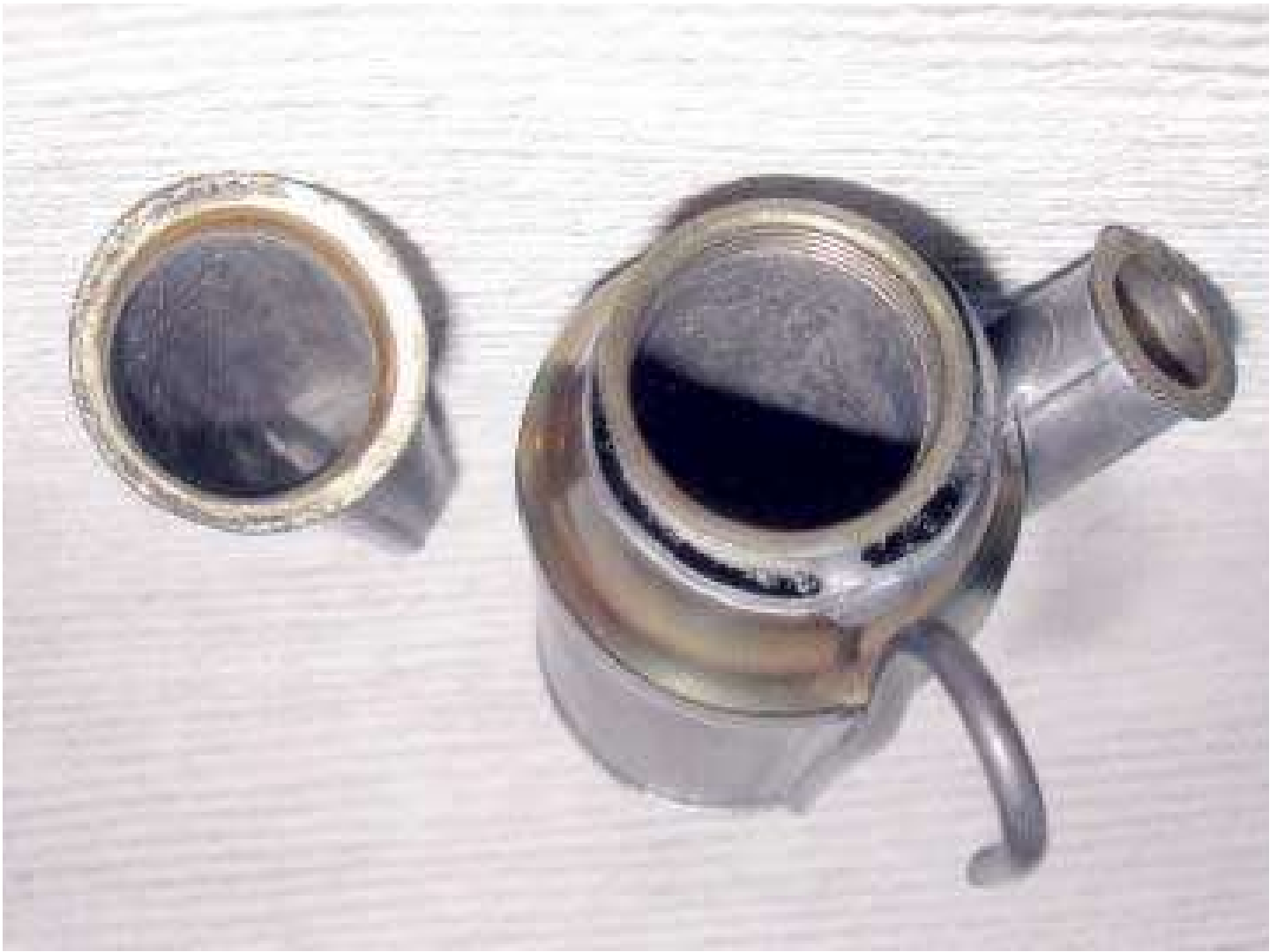
Figure 14: H. J. Richards lamp. Note the fuel chamber surrounds the wick chamber and the fuel flows through small connecting channels.
