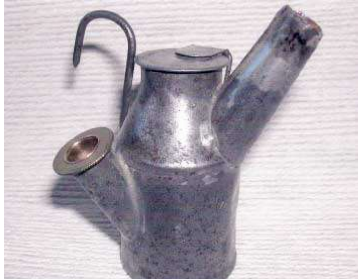
Figure 11: The Smythe lamp. Note the separate filler tube attached to the lower chamber and the hole for the smaller wick leading from the lower chamber to the upper main wick chamber.
