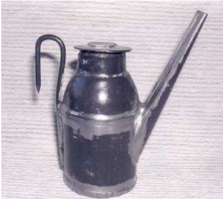
Figure 4: John Gable lamp with flattened spout. Claimed in patent that this controlled the flow of fuel.
