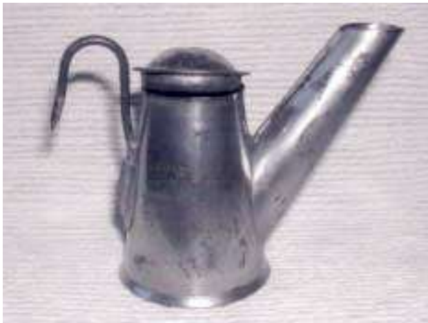
Figure 2: Jacob Vogele miner's face lamp. Note the domed lid with vent hole and the recessed bottom that would collect oil and return it to the font.
