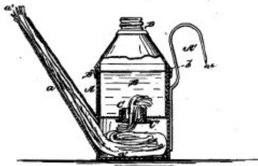
J. O. DAVIES, et. al.: Note that in this lamp the main fuel chamber is the upper chamber. This would appear to be more efficient.
