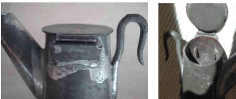
Figs. 7 and 8: The patented lid eliminates the vulnerable solder joint at the lid, and is further strengthened by having the lugs penetrate the font. Also note the protective cover soldered over the hinge lugs.
