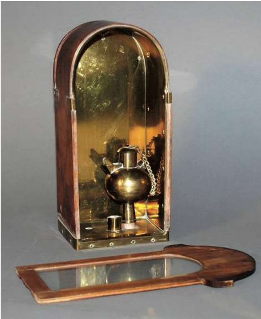
Figure 13. Freiburger Blende, late 19th-century, with spherical "coo-coo lamp" inside. Staatliche Kunstsammlungen Dresden, Grünes Gewölbe collection; Jürgen Karpinski photo.
