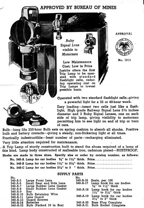
One lamp using dry cell batteries did see use in the mines. With weight not being an issue for mine car lights, Justrite Mfg. Co. produced a cast iron trip lamp powered by two D-cells. Ads have been seen as early as 1912 and it was listed in Justrite catalogs into the 1930s. In a manner similar to safety lamps used for testing gas, a special key (kept outside the mine) was needed to open the lamp since an electric spark could also ignite methane.
