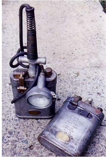
George and John Oldham both Engineers were interested in improving and simplifying the construction of the lamp so that the contacts and other parts can be easily and quickly repaired and maintained by unskilled workers without special tools making the lamp more economical and convenient.
