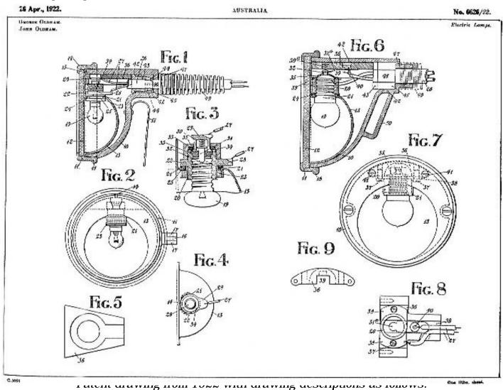
Figure 1 is a sectional side elevation of a suitable construction of the lamp.
