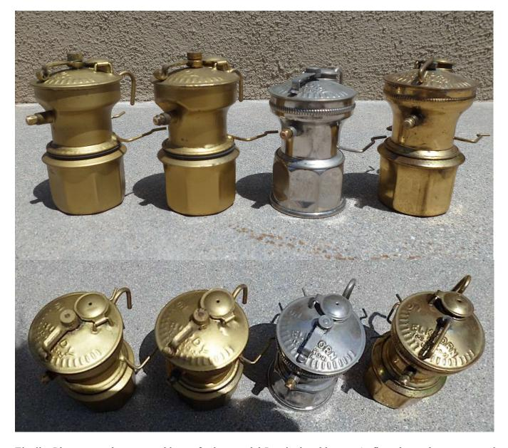
Finally, I have come by two steel bases for late model Justrite hand lamps. At first glance they appear to have brass lids. But these "lids" have uncrimped edges and predrilled holes — they are in fact the unassembled lower portions of water tanks.
