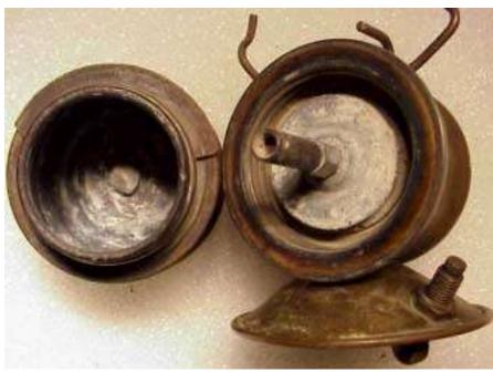
Details of the double gasket mechanism. A standard Britelite gasket is a perfect match for the outer gasket. Note the tiny knurled adjustment knob at the end of the striker.
