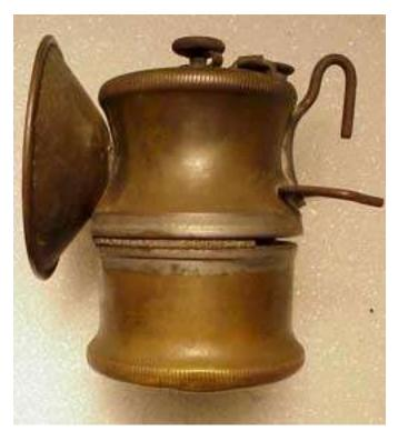
The reflector is heavy spun brass and screws onto a threaded gas tube. There is no reflector brace, but a lock-nut holds it firmly in place. The lock-nut perhaps also served to allow precise positioning of the striker.
