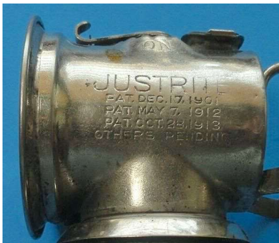
Left: Justrite Jiffy tank showing parabolic crease encroaching onto "OTHERS PENDING." Also note high shoulder beneath water lever. Right: Standard horizontal lamp with crease below stamp mark.
