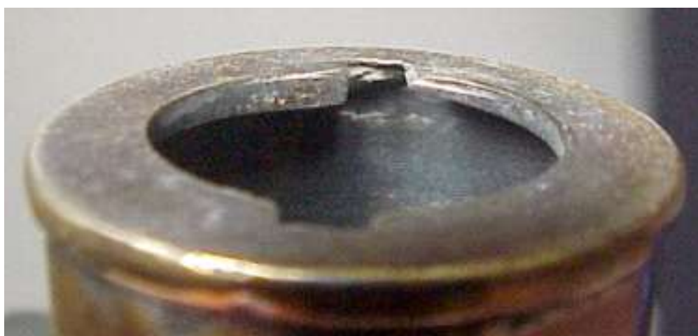
Top of base showing bevel for cam lock.
