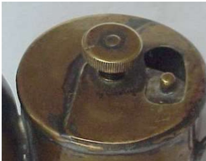
Top view of lamp showing sliding waterdoor closed and open.
