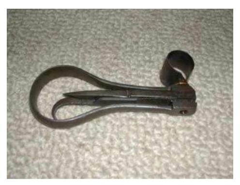
This folder (7.5--4.5in) was found in Retallack's Colorado home and originally acquired by Leo Stambaugh. The Retallack hook incorporates a knife edge cutter while the spike has both a serrated cap crimper and fuse cutter indentation.
