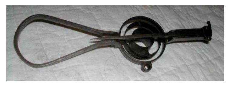
The spike folds neatly into the handle and keeps the gimbal from rattling about. The last photo compares the "Folding Gimbal" to two of the patented Gimbals; ie: the Rasmussen (patented 1903) and the Weed (patented 1906). If the candlestick does anything, it illustrates the amazing effort of our forefathers to develop a better widget.
