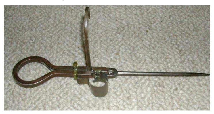
An early and crude prototype of the patent was first developed by Werntz prior to his patent. The thimble of the prototype is attached by means of a sliding brass post and the hook, when disassembled is secured by a sliding square brass socket. Because of the various deficiencies for practical use the prototype was probably quickly scrapped as Werntz went on to develop his patent model. The prototype is illustrated below.
