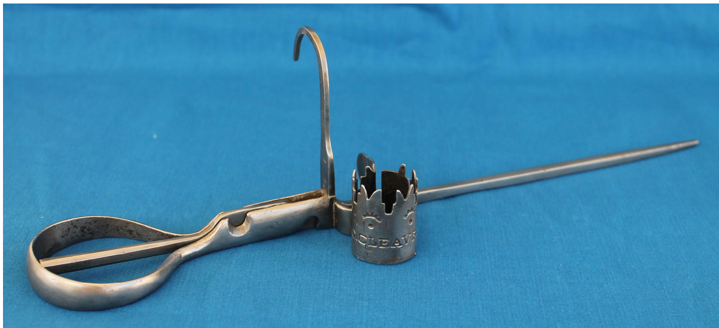
Fig. 8 - C. Cleaves fuse cutter candlestick in its closed position (thimble side) after restoration.
