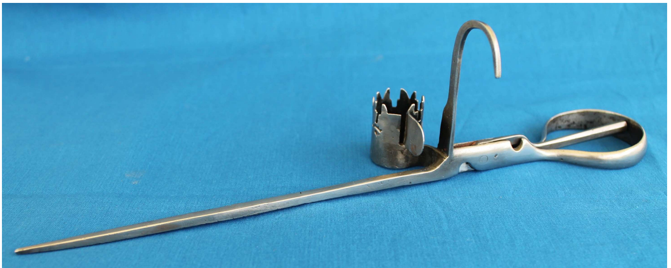
Fig. 11 - C. Cleaves fuse cutter candlestick in its closed position (hook side) after restoration.
