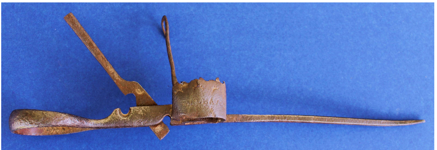
Fig. 3 - C. Cleaves fuse cutter candlestick in its open position (thimble side) before restoration.
