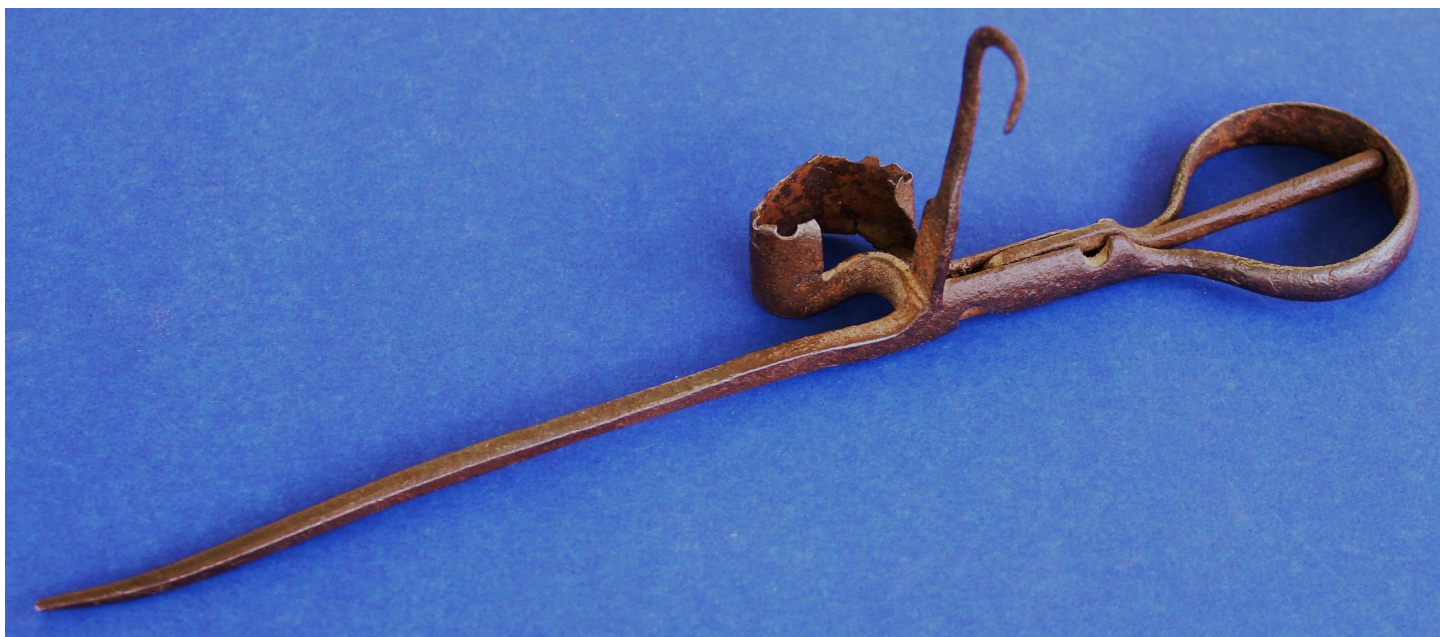
Fig. 4 - C. Cleaves fuse cutter candlestick in its closed position (hook side) before restoration.
