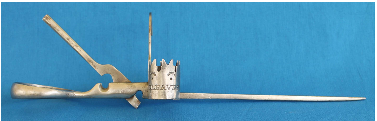
Fig. 10 - C. Cleaves fuse cutter candlestick in its open position (thimble side) after restoration.
