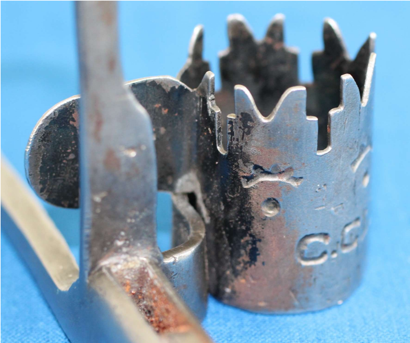
Fig. 12 - C. Cleaves fuse cutter candlestick thumb lever and thimble with corrected “C” after restoration.
