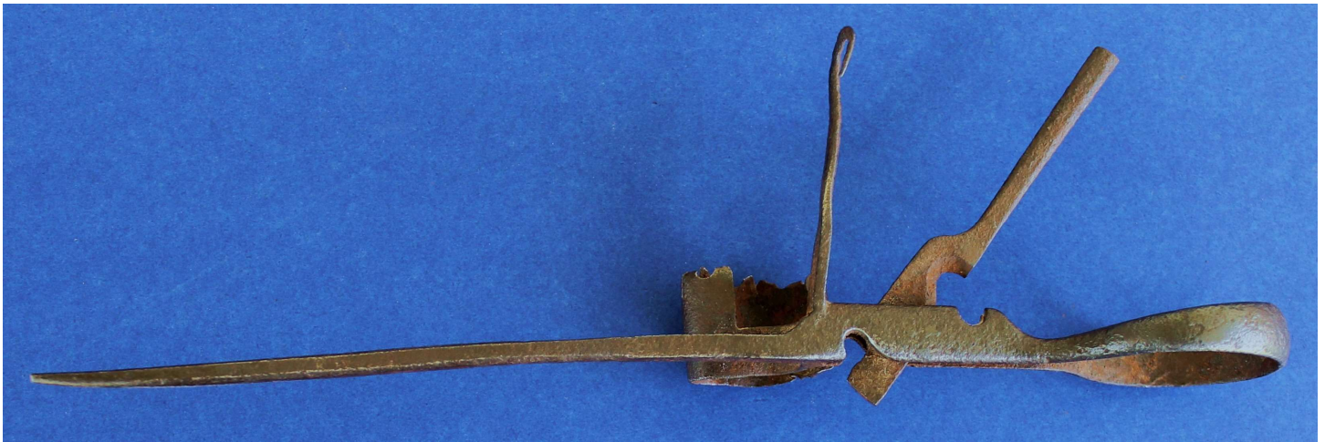
Fig. 2 - C. Cleaves fuse cutter candlestick in its open position (hook side) before restoration.
