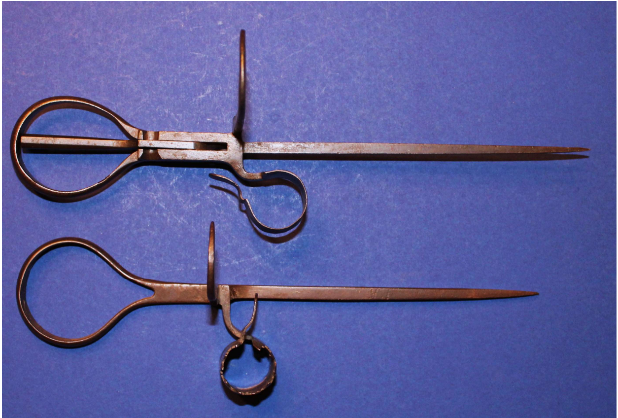
Fig. 8 - C. Cleaves fuse-cutter & standard stick. A view showing the relationships of the thumb tabs to the hooks as seen from above.
