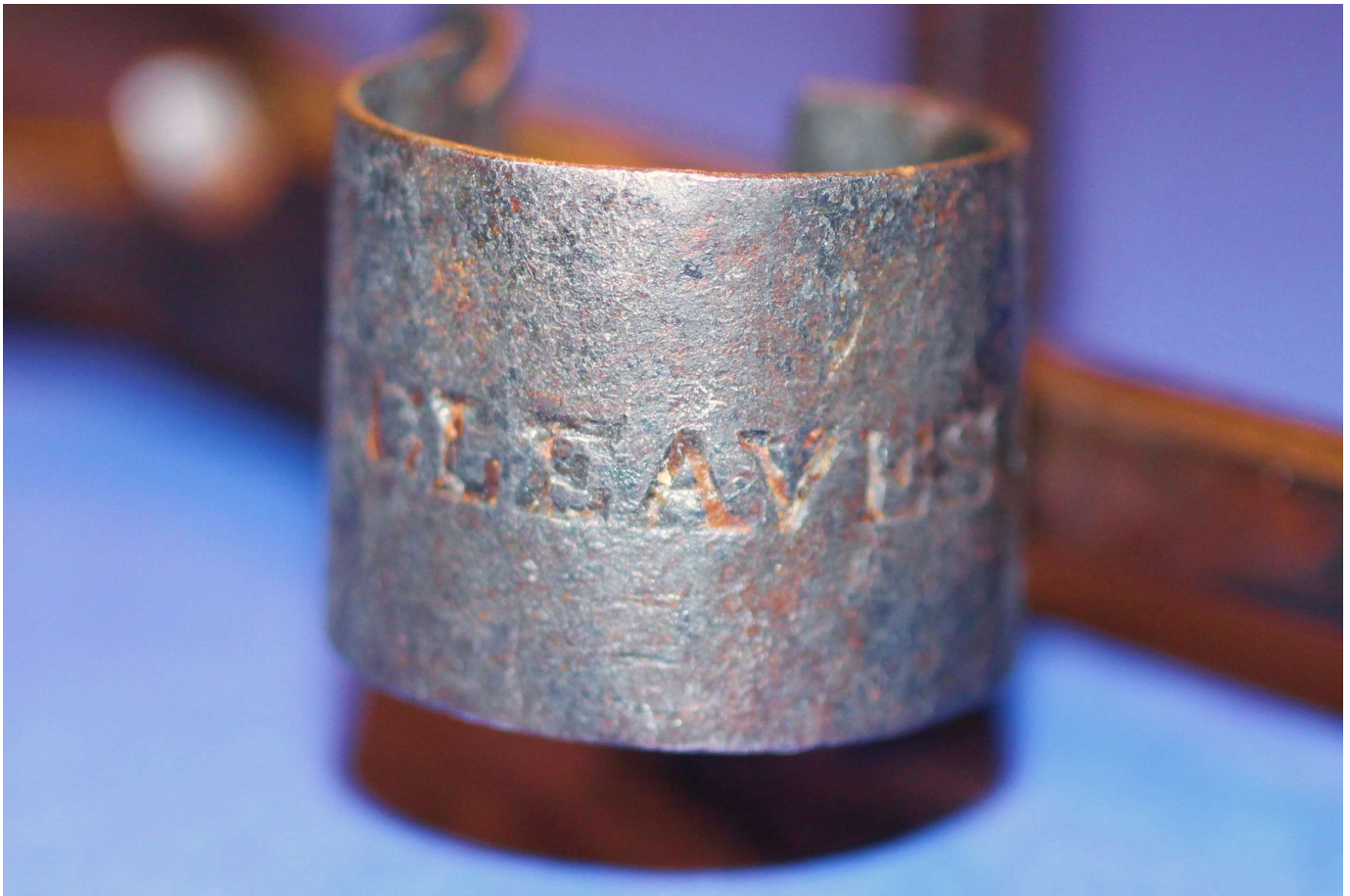
Fig. 3 - C. Cleaves fuse-cutter thimble: very plain without castellations.
