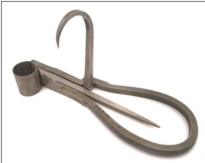
Hook in the reverse position for folding down into the handle.
