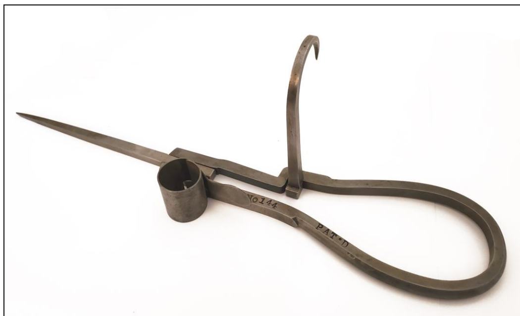
Candlestick fully unfolded, with the hook twisted into the locked position
