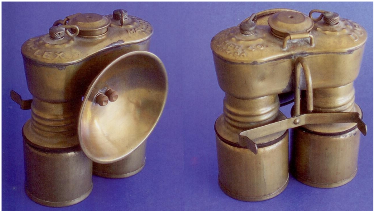
Front and the back views of a Maumee Duplex Carbide Lamp. Courtesy, Dave Thorpe
