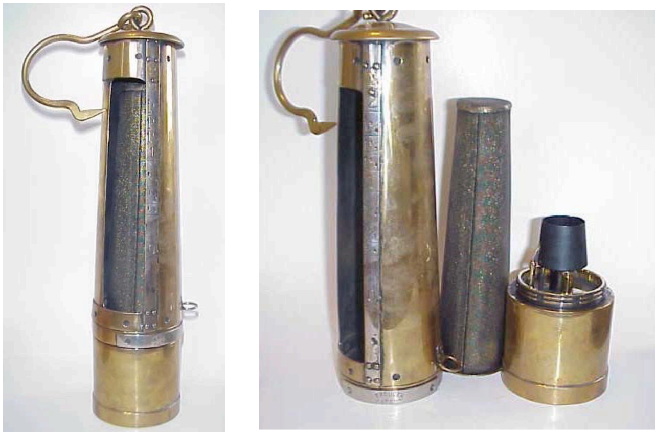
Figure 11: All brass Pieler made by Joesef Jermar, Ostrau. Sliding bonnet with scale that measures up to 2 1/4% methane. Magnetic lock marked “Broucek Patent”. Wick “snuffer.”
