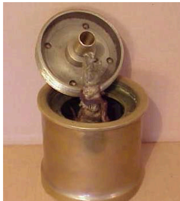
Figure 2: (above and right): This is Pieler's original design, but with scales added. The gauze is steel with a copper cap similar to a Saarbrücken lamp. The font is complex because of having to facilitate the hollow tube that runs from the bottom of the lamp through the center of the burner. Circa 1887.
