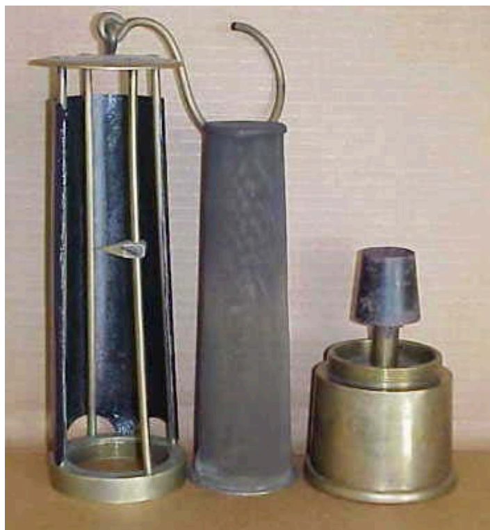
Figure 4: Early Friemann & Wolf Pieler. Serial #46710; circa 1888. No fixed scale. Notice that the lamp has a pointing device that slides up and down one of the standards for marking the height for the flame. No igniter or flame snuffer.
