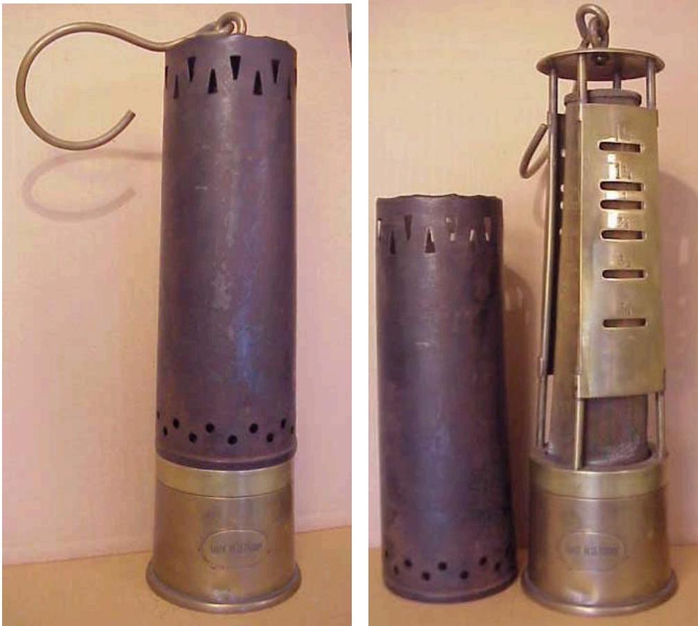
Figure 6: Friemann & Wolf Pieler. Serial No. 201711; circa 1895. Classic Pieler lamp with 2 scales. Fitted with removable bonnet to be used for traveling in mine with the lamp lit. Bonnet has no slot for flame observation, so bonnet must be removed prior to testing. No igniter or flame snuffer. This lamp was exported to America, and has a brass tag on the front that says “Made in Germany.”
