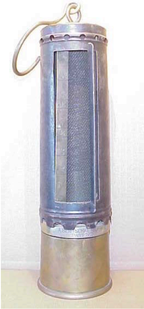
Figure 12: Benitschke's Sohn was a well-known manufacturer of mining lamps in what was Bohemia (Czech Republic region). This particular Pieler lamp is fitted with a removable bonnet that has a sliding window for observation.
