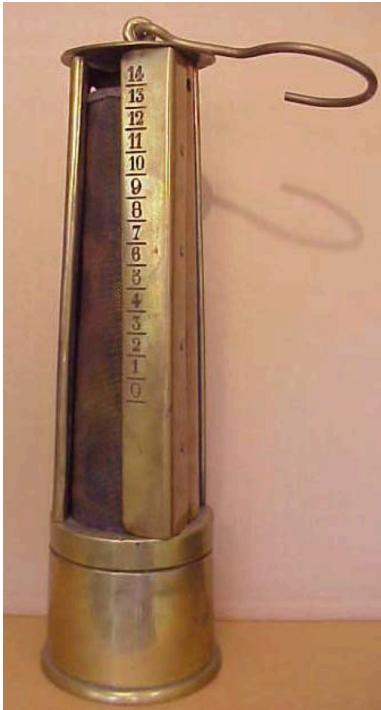
Figure 8: French Cosset-Dubreille Pieler. Notice scale measures length in centimeters, with no % methane indication.
