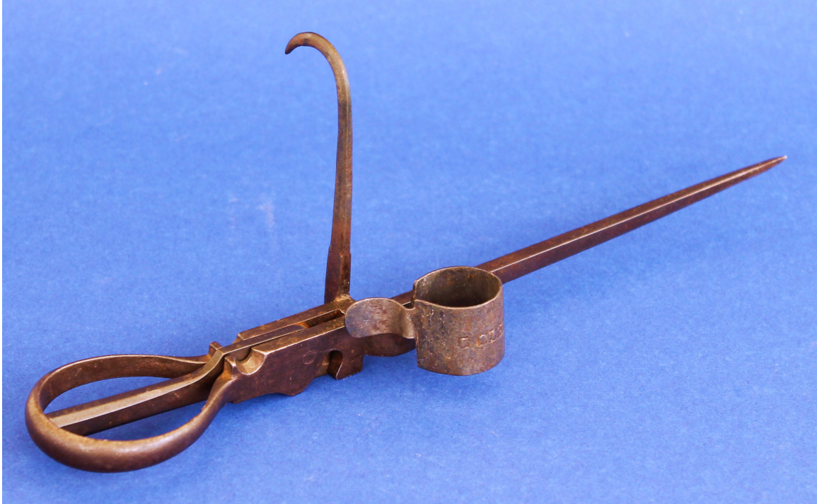
Fig. 1 - C. Cleaves fuse-cutter candlestick. The thimble side of the closed candlestick.
