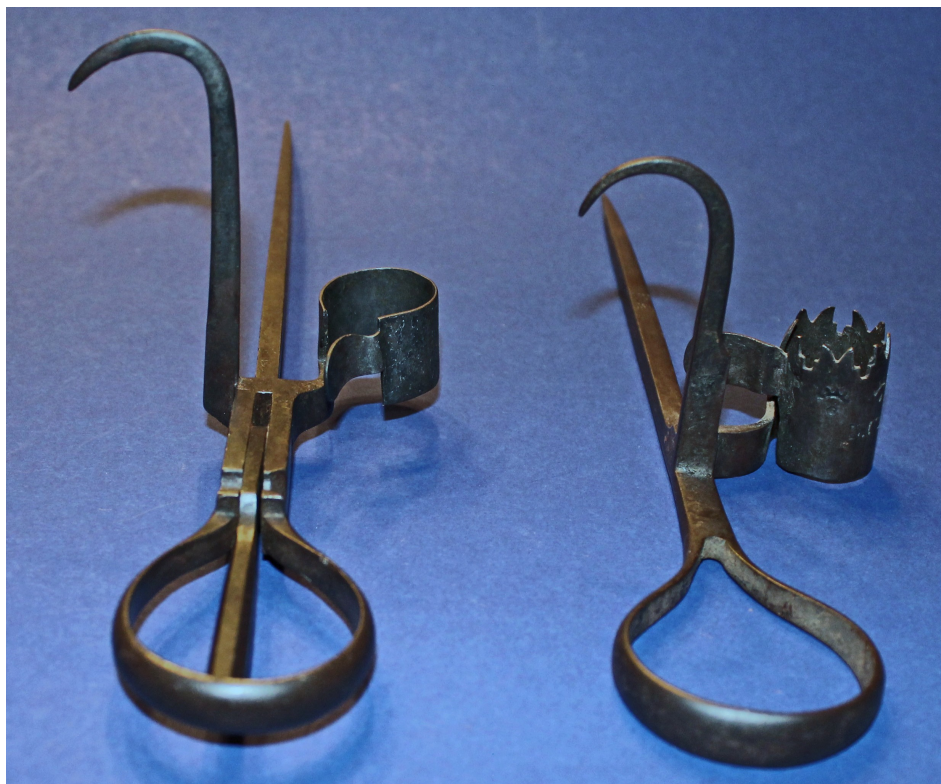
Fig. 7 - C. Cleaves fuse-cutter & standard stick. A view showing the relationships of the thumb tabs to the hooks as seen from the handles.
