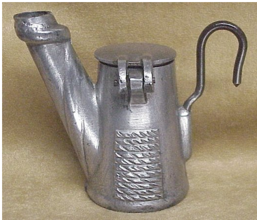
Above: Cast lamp with match striking surface and drip ring on spout.
