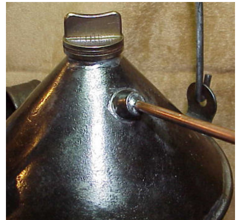
Above: Wolf Safety Lamp filler, brass name plate and vent tube.
