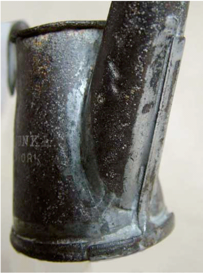
Funke's Indestructible lamp, John Leahy collection. Note the reinforcing bar that is an inverted "T".
