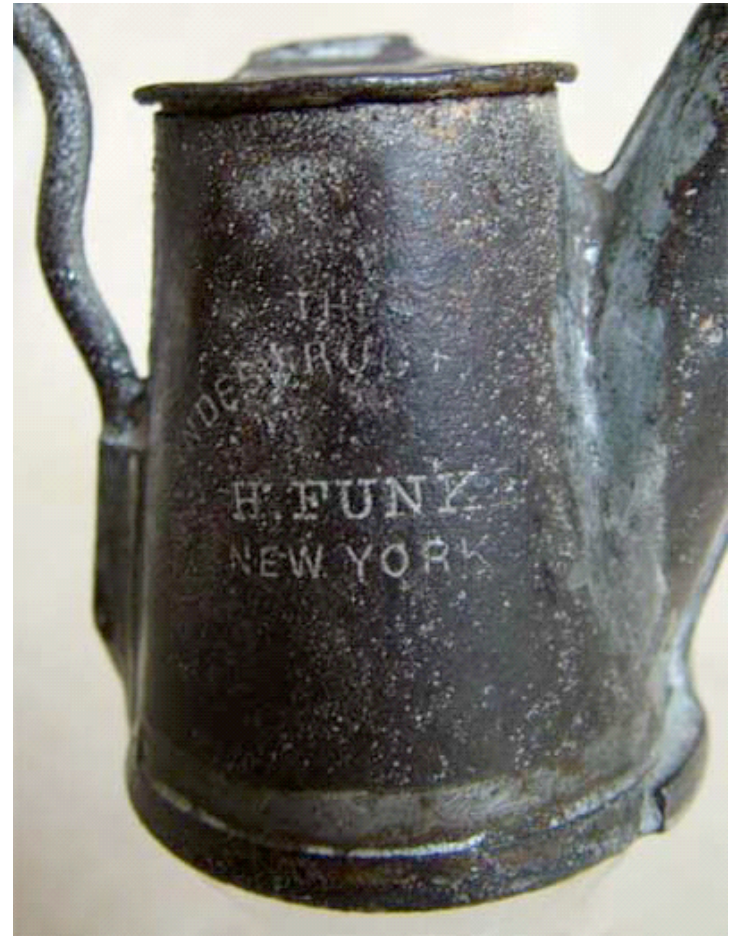
Funke's Indestructible lamp, John Leahy collection. Note the reinforcing bar that is an inverted "T".
