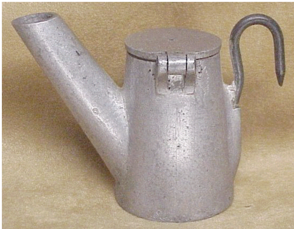
Above: A small cast aluminum lamp that is identical to the NO MELT, but without stamping.
