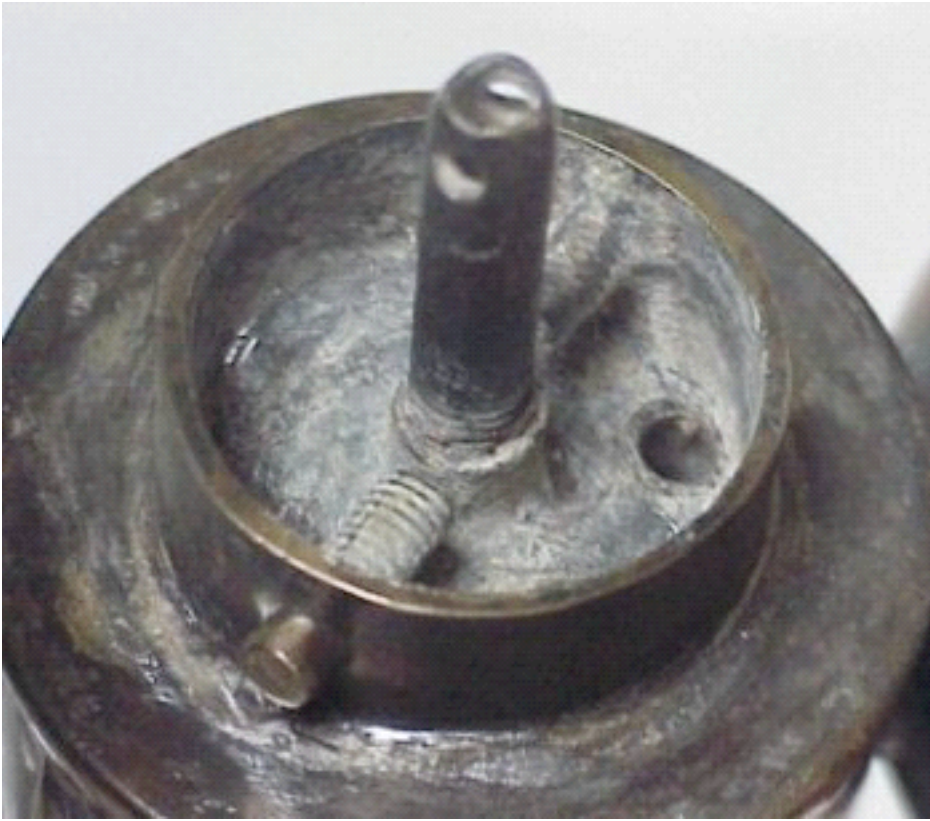
Left: underside of water chamber showing cam pins.
