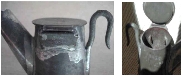
Figs. 7 and 8: The patented lid eliminates the vulnerable solder joint at the lid, and is further strengthened by having the lugs penetrate the font. Also note the protective cover soldered over the hinge lugs.
